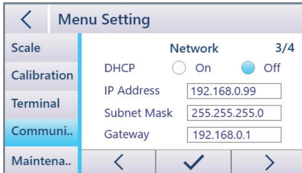
8. Enter an IP address for the scale, then press ✓ to confirm, then press < on the upper left corner to save the changes. To test the network connection, continue with step 9.
