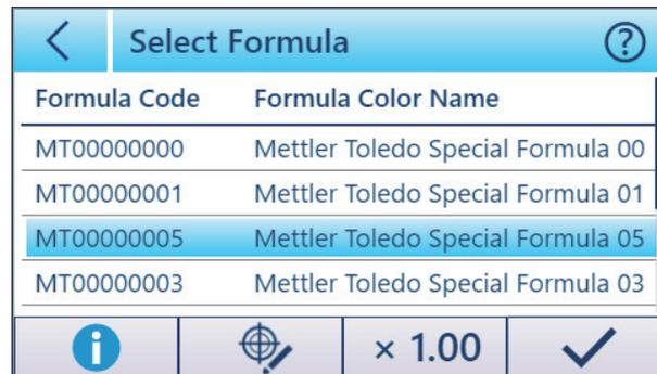
2. Press the Times button  $\times 1.00$  to toggle between target amount values of  $\times 0.20$ ,  $\times 0.50$ ,  $\times 0.75$ ,  $\times 1.50$ ,  $\times 2.00$ ,  $\times 3.00$ ,  $\times 4.00$ ,  $\times 5.00$ .
